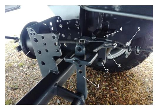
Figure 19.The components of the brake system:1 - expander roller lever, 2 - adjusting nut, 3 - expander roller, 4 - brake equalising bar,<br/>5 - parking brake cable, 6 - cylinder
