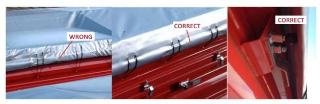
Figure 3. Correct tensioning of the tarpaulin cover
